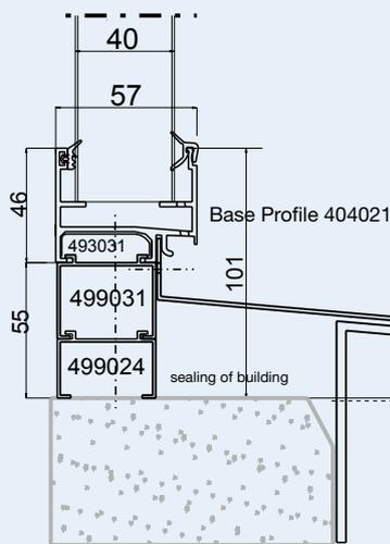
Base profile 404021 and adapter profiles 499024 and 499031 for windowsill projections from 320 to 360 mm
