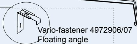
For projection/profile depth of more than 150 mm additional Fastener (Vario-fastener or Clinker-fastener) are necessary on the structure (every 800 to 1,000 mm) Aluminium windowsills should project approx. 40 mm about the ready facade. Accordingly the profile width needs to be measured. This is only valid if side end pieces are installed as well. Without side end pieces the windowsill must project 20 mm over the ready facade (refer to 1.2.10.2)
