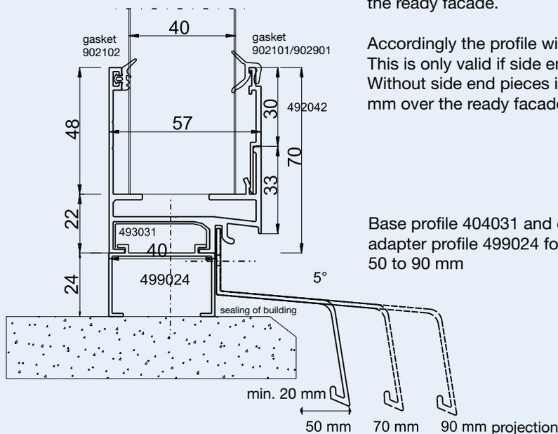
Base profile 404031 and clamp batten 492042/43 with adapter profile 499024 for windowsill projections from 50 to 90 mm
