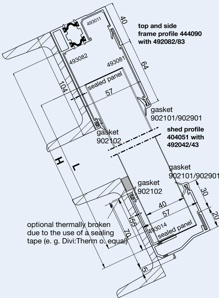
Calculation of panel length:  $L$  in mm = Height  $H$  in mm - 75 mm
