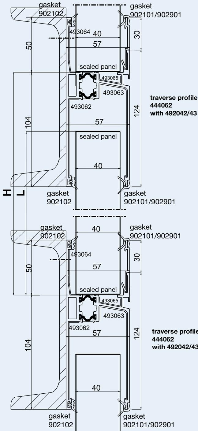
Calculation of panel length:  $L$  in mm = Height  $H$  in mm - 65mm
