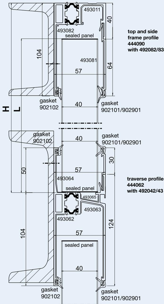
Calculation of panel length:  $L$  in mm = Height  $H$  in mm - 65 mm
