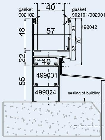
Base profile 404031 and clamp batten 492042/43 and adapter profile 499024 for windowsill projections from 320 to 360 mm
