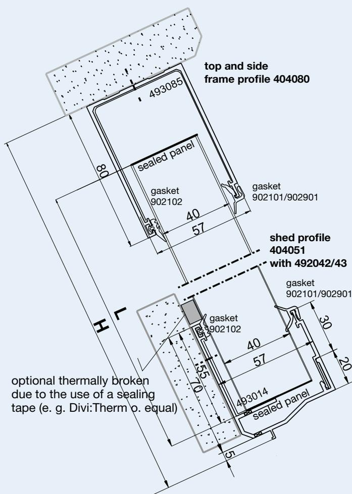
Calculation of panel length:  $L$  in mm = Height  $H$  in mm - 75 mm
