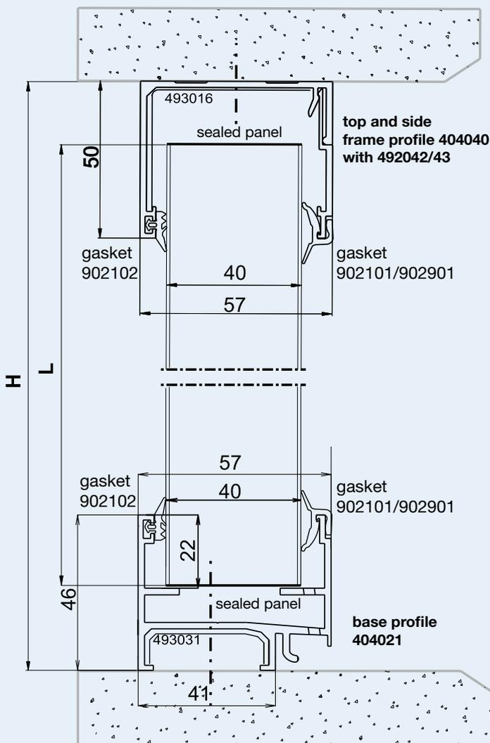
Calculation of panel length **L** in mm = Height **H** in mm - 50 mm
