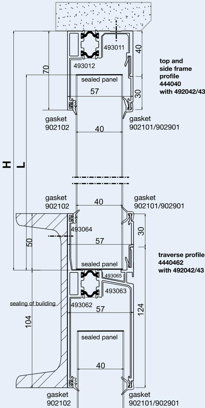
Calculation of panel length:  $L$  in mm = Height  $H$  in mm - 50 mm
