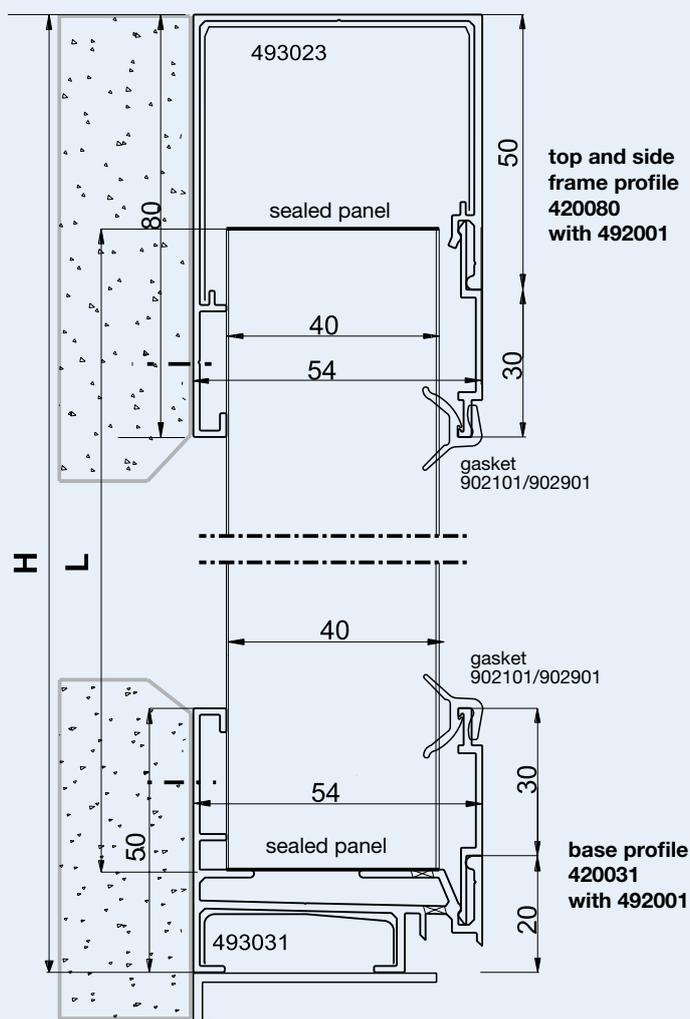
We recommend to support the base profile for panel length starting from 6.00 m.
