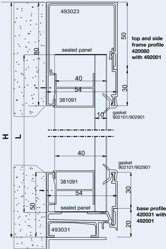
We recommend to support the base profile for panel length starting from 7.50 m.
