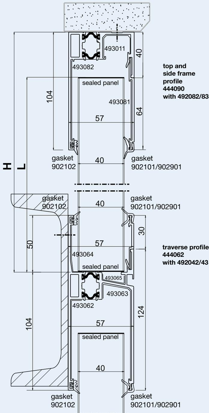
Calculation of panel length:  $L$  in mm = height  $H$  in mm - 65 mm
