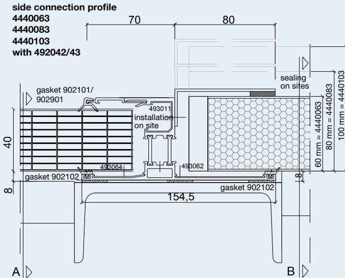
Distance of substructure to PC panel 8mm
