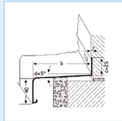
Aluminium windowsills should project approx. 40 mm over the ready facade. Accordingly the profile width needs to be measured. This is only valid if side end pieces are installed as well. Without side end pieces in place the windowsill must project 20mm over the ready facade. (refer to 1.2.10.2)
