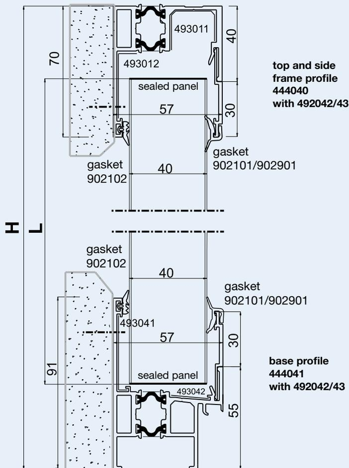
Calculation of panel length:  $L$  in mm = Height  $H$  in mm - 90 mm
