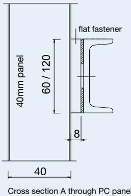
Cross section A through PC panel
