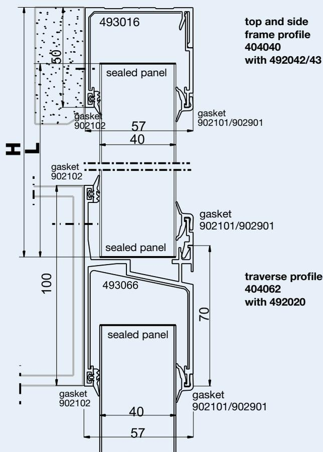
Calculation of panel length: **L** in mm = Height **H** in mm
