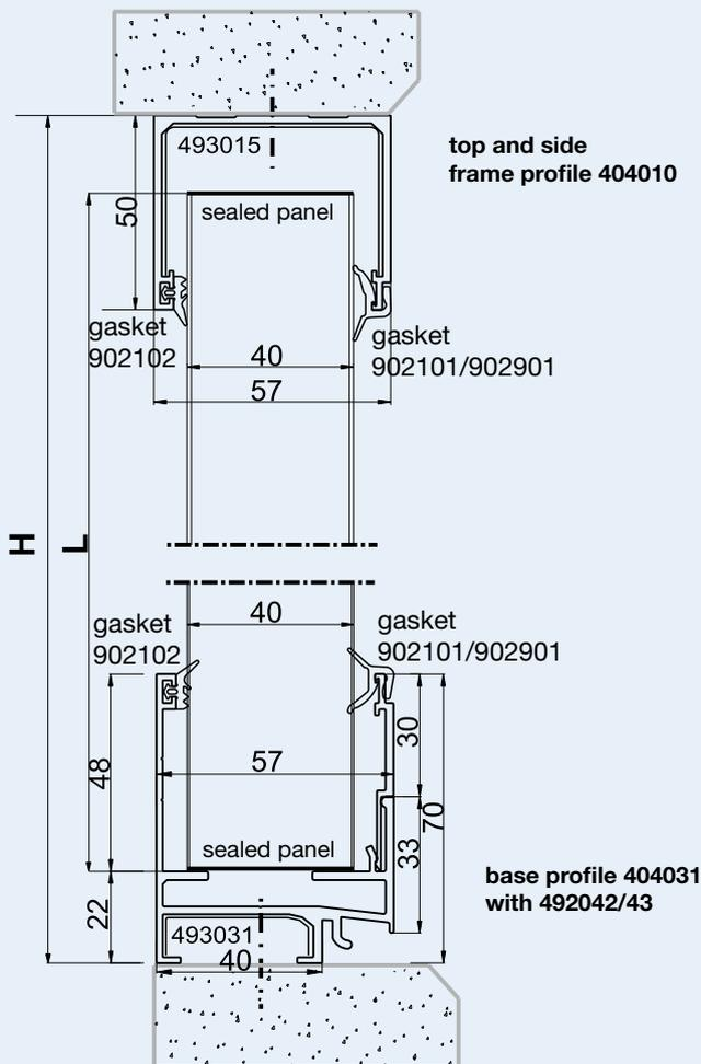
Calculation of panel length:  $L$  in mm = Height  $H$  in mm
