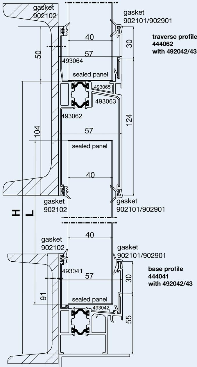
We recommend to support the base profile for panel length starting from 7.00 m
