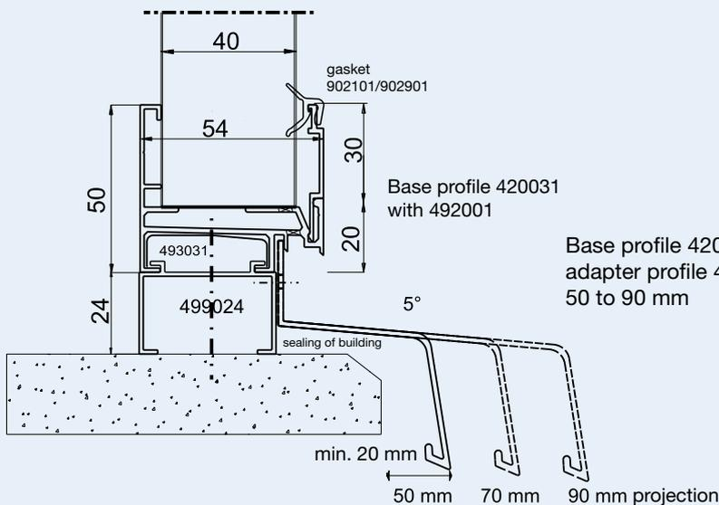
Base profile 420031 and clamp batten 492042/43 and adapter profile 499024 for windowsill projections from 50 to 90 mm
